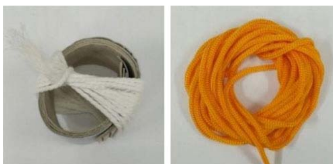
Fig. 2 Subjects of the test: Cot (left) and PP strings (right).
